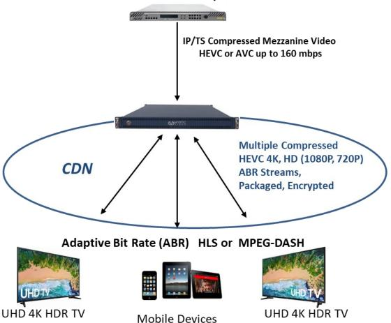
The platform supports transcoding of mezzanine video feeds of up to 100 mbps each into multiple HD and 4K resolutions compressed with HEVC/H.265 or AVC/H.264
